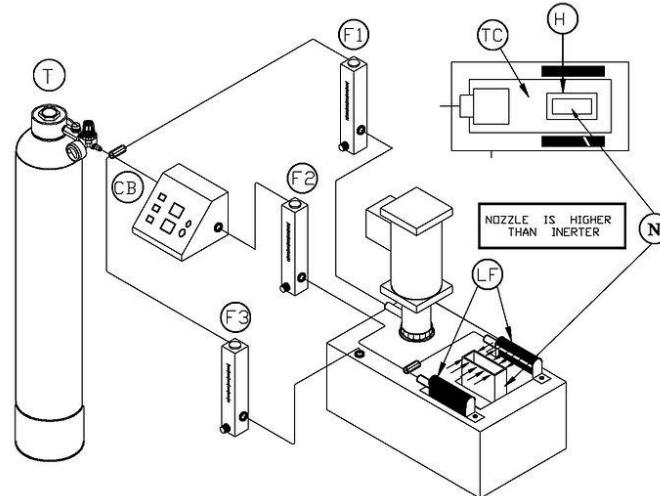
(T) Nitrogen tank (or plant nitrogen supply) with regulator and gauge
