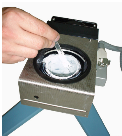
Picture A. Silicone paste application
