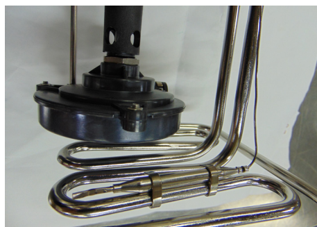
7.6a Thermostat bulb for working at temperatures below 120°C
