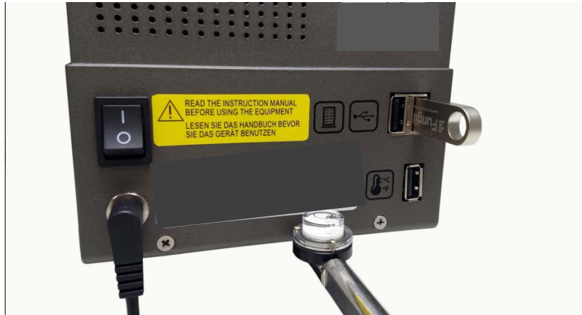
Fig. 7 USB-memory stick connection
