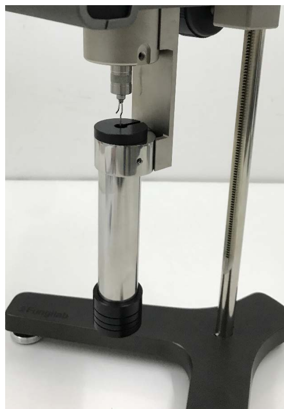
Fig.8: LCP Adapter assembled in viscometer
