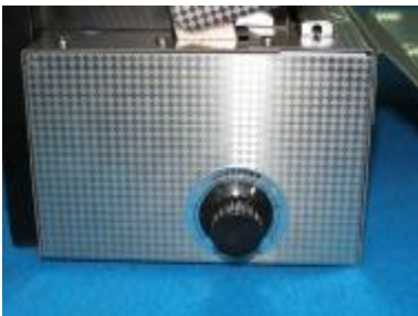
Sealing temperature selection knob.
