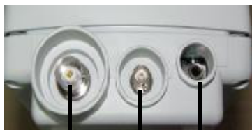
Electrode pH Temperature probe Output RS-232
